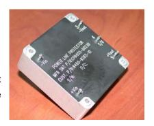
The products protect electronic instruments against transients, surges and voltage fluctuations that are inherent in military land vehicles (as described in MIL-STD-1275).
